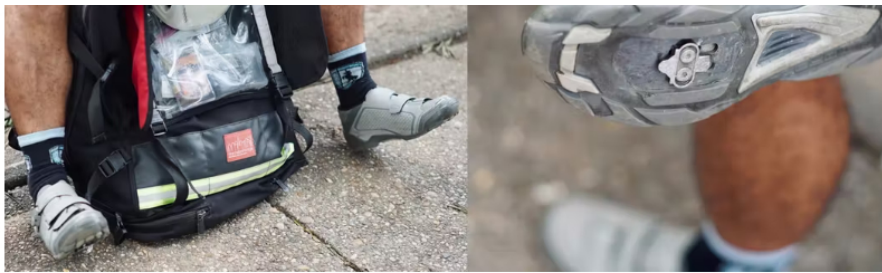
Shimano SPD pedals combined with MTB shoes a top choice with bike couriers. This rider admitted they started out wearing road shoes and quickly learned how dangerous it was to be walking around in them. Photos by Jacob Cummings
